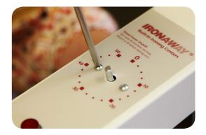
Using a Phillips screwdriver, remove the two screws on the sides of the timer face (where the knob was).
