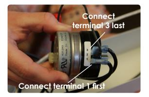
Connect raceway wires to new timer by first connecting long black wire to terminal marked 1. Then connect the shorter wire to terminal marked 3.
