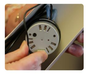
Place shaft of new timer through hole in raceway with the three terminals on top pointing towards back of spotlight.
