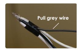
Unscrew the wire nut on bundle of white wires by twisting nut counterclockwise. Locate the dark grey wire that connects to timer and remove from bundle by gently pulling it.
